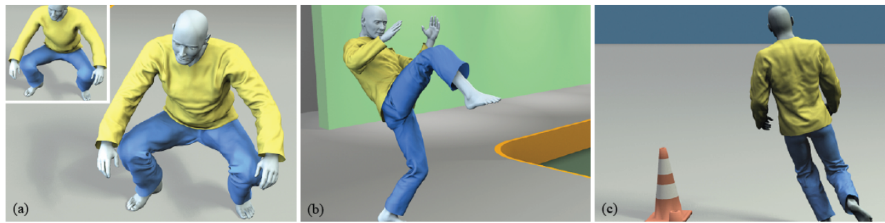
Figure 4: The method of [Wang et al. 2010] uses a precomputed dataset to synthesize cloth wrinkles (a) that are layered onto a coarse base simulation (inset). The precomputed dataset can be used to synthesize wrinkles for a wide range of poses (b and c).
